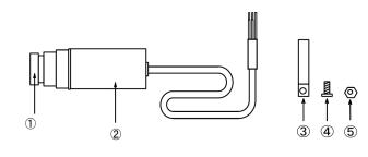
①Lens (Upper: Type G3.8) 2WAT-240E ③Installation ring mount ④ Screw for ring mount (M2.6 x 8mm) (5)Nut for ring mount (M2.6)
