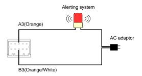
When connecting to the induced load(relay, motor) or incandescent electric lamp, take measures against surge voltage and inrushing current on the outside circuit.
